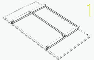
The mounting structure is rotated and opened on the other side of the arrow as shown below, loosen the fastening bolt of the expandable rod, as shown in the figure below, the arrow moves the expandable rod to the desired angle ( $10^{\circ}$ - $30^{\circ}$ ,  $40^{\circ}$ ,  $50^{\circ}$ ,  $60^{\circ}$  corresponds to 4 scale marks), adjusts the expandable rod to the corresponding scale and tightens the M8\*20 bolt.
