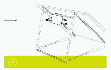
The mounting structure is rotated and opened on one side by the arrow as shown below, loosen the fastening bolt of the expandable rod, as shown in the figure below, the arrow moves the expandable rod up and down to the desired angle ( $10^{\circ}$ ,  $20^{\circ}$ ,  $30^{\circ}$ - $40^{\circ}$ ,  $50^{\circ}$ ,  $60^{\circ}$  correspond to 5 scale marks), adjust the expandable rod to the corresponding scale and tighten the M8\*20 bolt.
